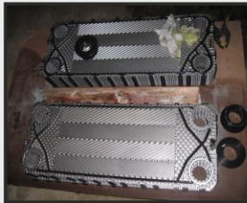
Plate heat exchanger
